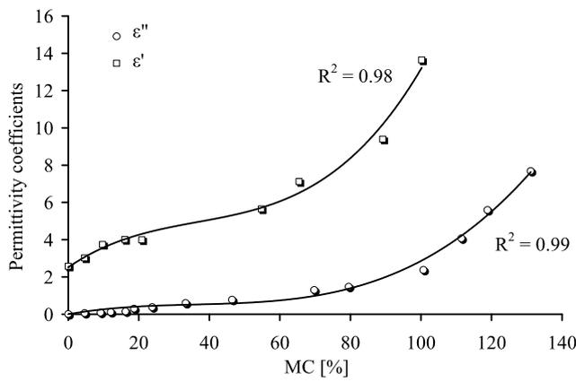
**Fig. 2** Permittivity coefficients as a function of *MC*
