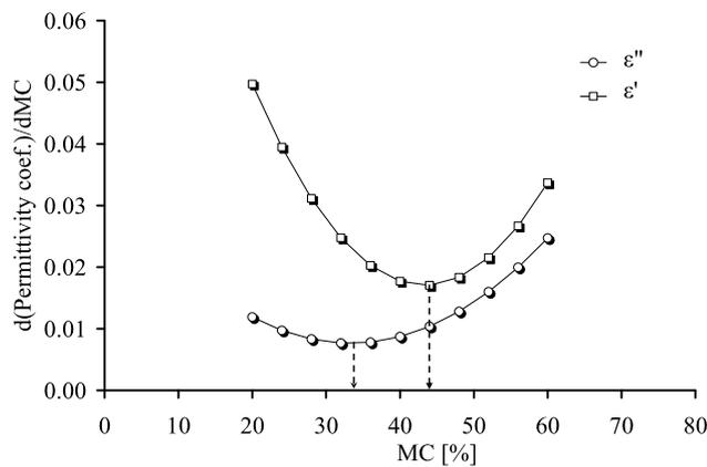
**Fig. 3** Sample plots of the derivative of the imaginary ( $\epsilon''$ ) and real ( $\epsilon'$ ) permittivity coefficients and how the *MC* associated with a change in slope was determined (*dotted arrow lines*)
