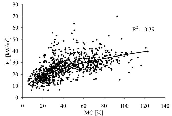
**Fig. 9**  $P_D$  versus  $MC$  for all experiments
